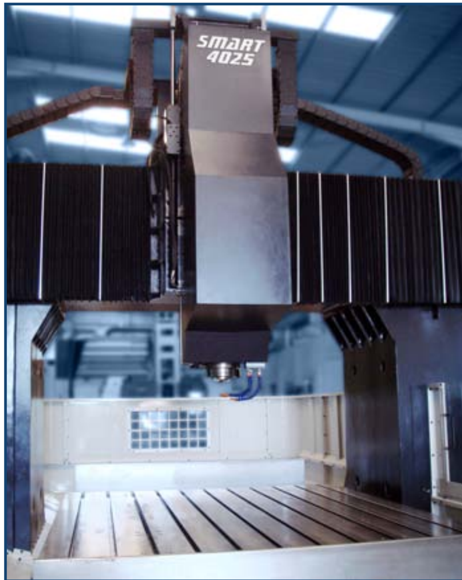
Z-Axis way system features a combination of Linear Guide-Ways and a Hard Box-Way for maximum rigidity
