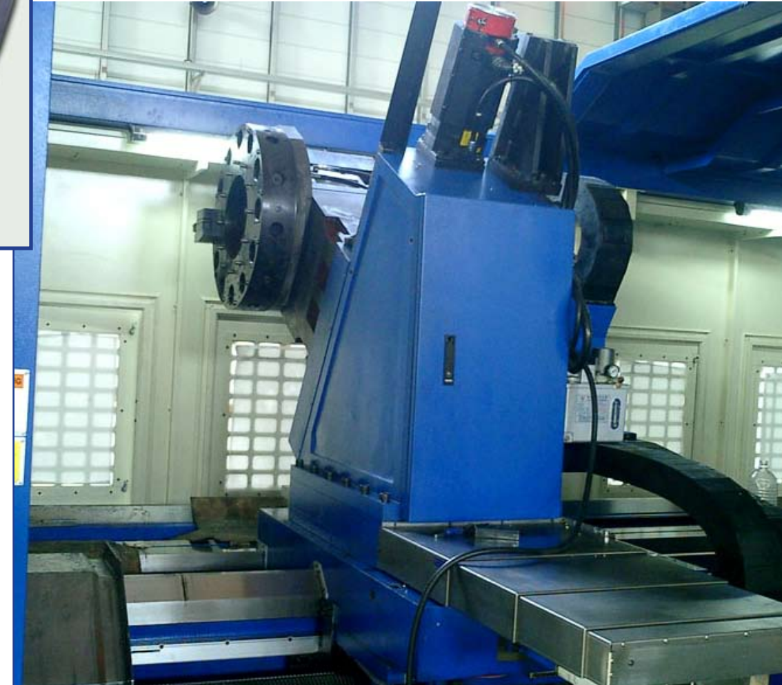
Live-Tooling with C-Axis and Y-Axis
