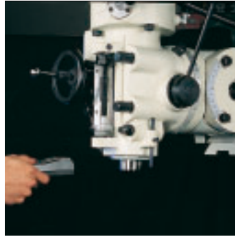
Spindle Running Noise Measuring less than 73 db at 1 meter
