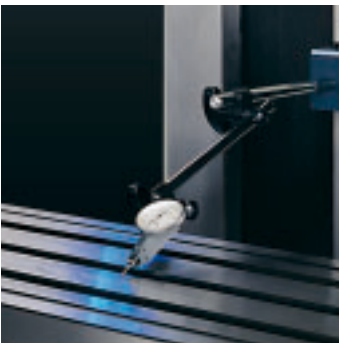
Parallelism of Table Surface to Table Longitudinal Movement less than 0.0008" per 20" of travel
