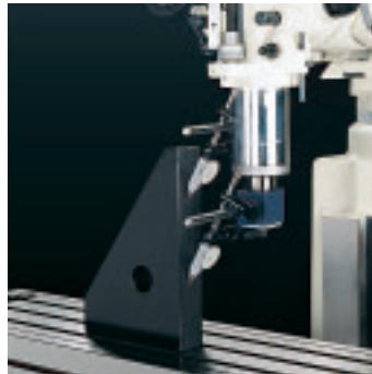
Squareness of Table Surface to Quill Travel less than 0.0008" per 5" of quill travel
