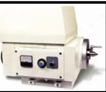
The Heavy-duty Meehanite cast workhead features an 8 piece precision angular contact bearing set and state-of-the-art electronic variable speed spindle drive. The combination live and dead type spindle allows for quick change from chuck to live center setup or vice-versa. The workhead swivels 90° counterclockwise and 30° clockwise for versatility.
