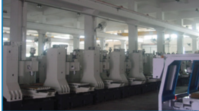
Heavy-Duty SMART Meehanite Castings on the assembly line
